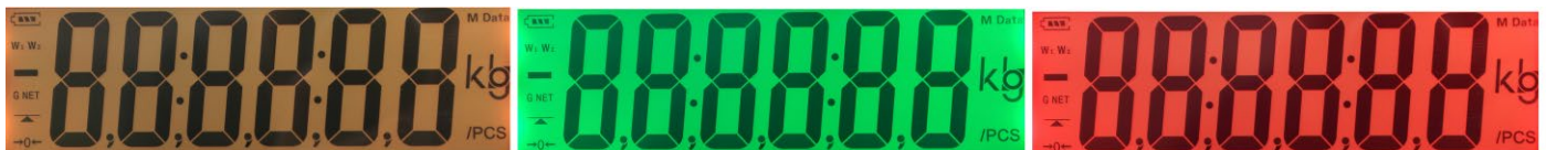
Adjustable Tri-Color Check Result Backlight
